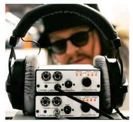
The front of the monotor has four headphone output jacks, two 3.5mm and two 1.4". The two jacks to the left are fed by one stereo amp and the two jacks to the right are fed by a separate stereo amp. For the bast performance use one set of phones per stereo amp output. But if you need to use all four, you will not damage the monotor and performance differences for casual use is minimal.
