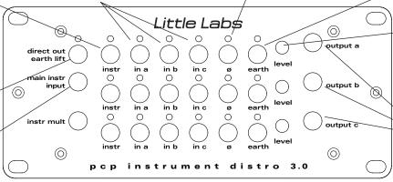
Pushing this button reverses the phase of the instrument impedance / level output (located to the right of each row of buttons on the front panel). Use it to eliminate phase (polarity) differences between different head or cabinets.
