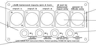
Use only the 48vdc 250ma power supply supplied with the PCP and plug in its 4 pin XLR here.
